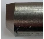
• A spindle roughing gouge should be sharpened square across with a single bevel, typically 45°.
